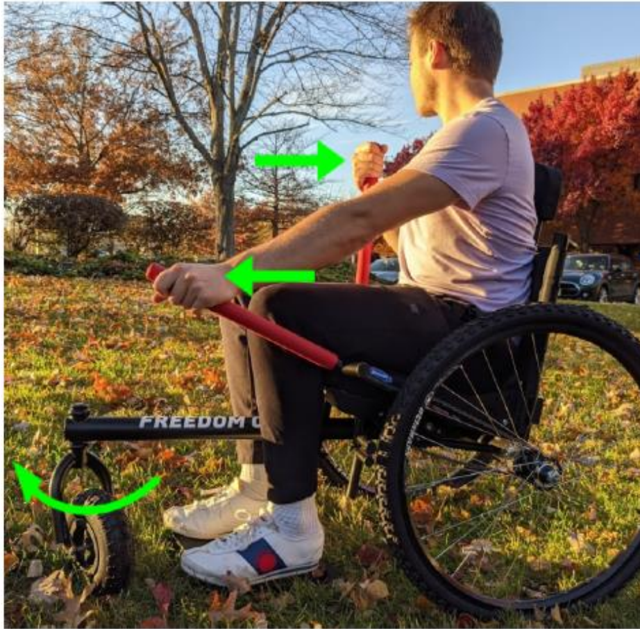
a) To turn right, apply the brake with the right lever and push the left lever forward.
